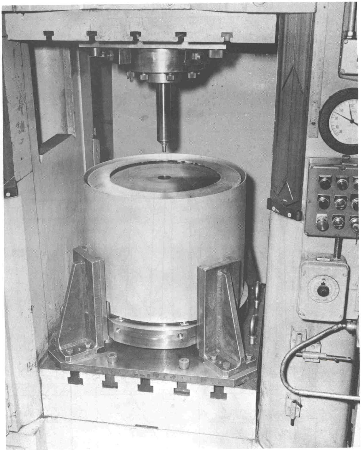
FIGURE 4. HYDROSTATIC-EXTRUSION TOOLING INSTALLED IN 700-TON VERTICAL HYDRAULIC PRESS AT BATTELLE
